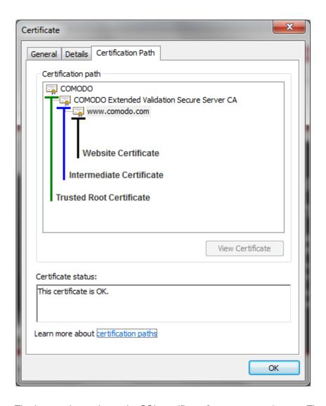
The image above shows the SSL certificate for www.comodo.com. The certification path shows the chain of trust that the browser uses to verify the certificate. The trusted root certificate has signed the Intermediate certificate which has in turn signed the Website certificate (the one for www.comodo.com).
